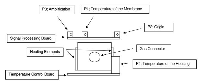
The setting of the potentiometer P1 depends on the application (gases and ranges) and should only be changed by personnel who is familiar with the FTC110 detector.
