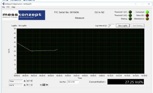
The Main Chart is the main window for reading measurement values, saving data, adapting the scale in x (time) and y (value) direction.
